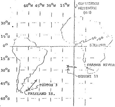
THE ARROWS ATTACHED TO THE X'S WHICH DEPICT THE LOCATIONS OF THE SATELLITES INDICATE THE APPROXIMATE DIRECTIONS OF MOTION WITH RESPECT TO THE FLAT MAP COUNDINATES (A MILLER CYLINDRICAL PROJECTION; DO NOT ATTEMPT A LINEAR DISTANCE MEASUREMENT FROM THIS MAP.)
