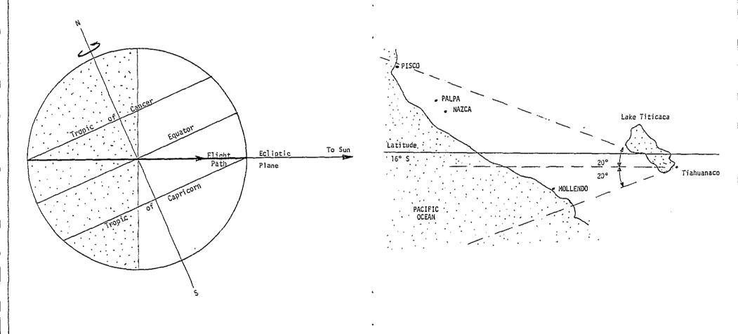
Fig. 1: Flight Path for Landing in Daylight Between Equator and Tropic of Capricorn at Summer Solstice in Southern Hemisphere from Orbit in Ecliptic Plane.
