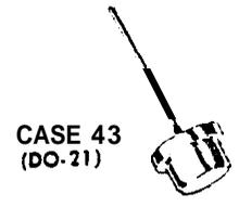
Medium-current silicon rectifiers - compact, highly efficient silicon rectifiers for medium-current applications.
